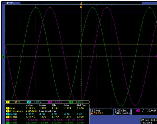
Fig. 8.4 Supply voltages in D-Q components for both Models
