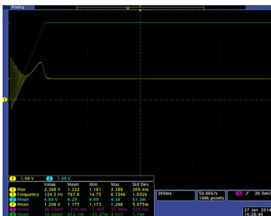
Fig. 8.6 Electro-mechanical torque (Yellow) and electrical rotor speed (Blue) healthy machine
